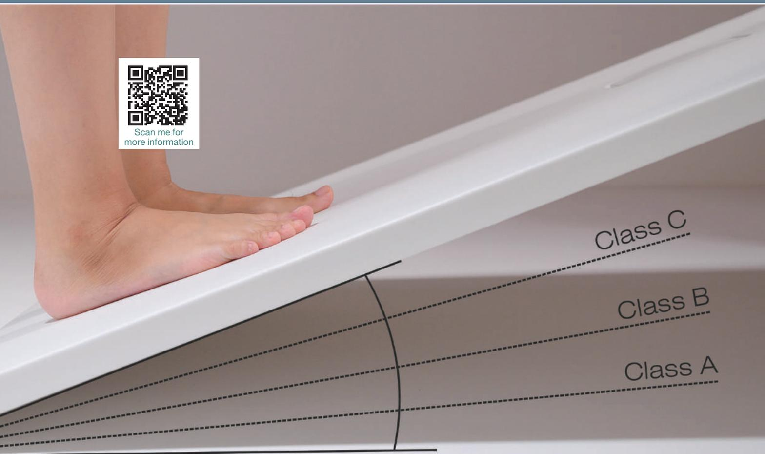
Exceeds Class C for DIN 51097 - Barefoot ramp test.
