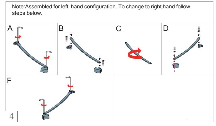
A.Position the bracing bar on the glass and against the wall.Make sure the bracing bar clamp is a minimum of 300mm from the edge and between 30-45 degrees to the glass.
