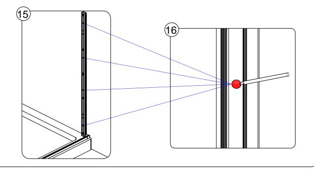
Remove profile and drill holes for wall brackets with diameter 6mm masonry bit and insert wall plugs. Make sure wall plugs are flush with tile.
