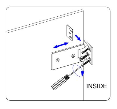
To remove bottom positioning aids open door outwards.
