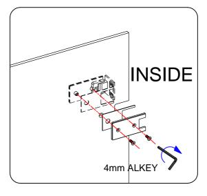
Place locating aids on threshold, one each side of opening. Lift door onto locating aids.
