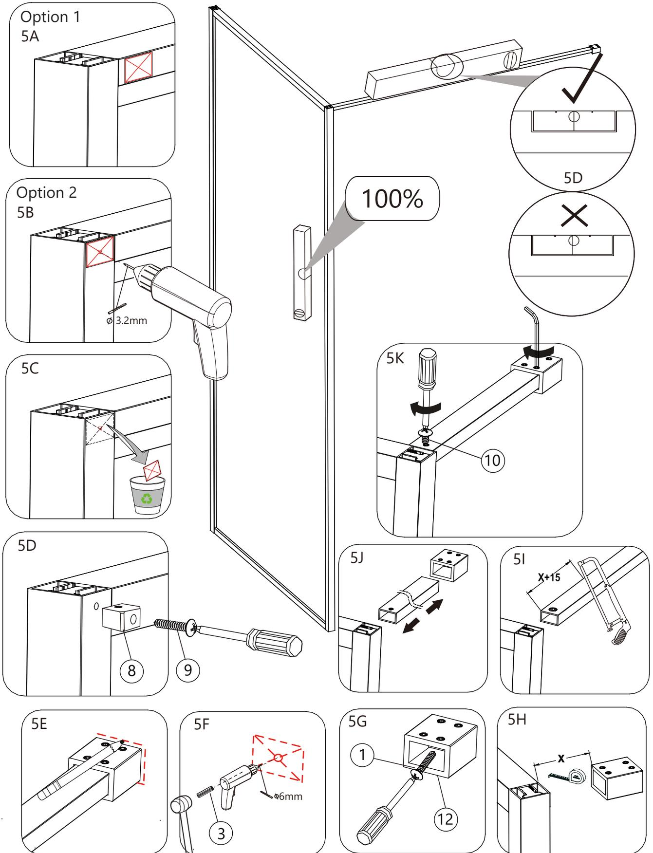
Adjust the shower enclosure ensuring it is level. Drill 4 equally spaced holes along the length of the wall profile to secure the shower wall.
