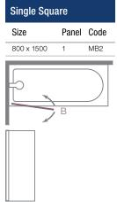
Door Swing: 90° in and out B: Radius of Screen Swing = 733mm □◯ Recommended shower head position
