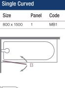
Door Swing: 90° in and out B: Radius of Screen Swing = 735mm C Recommended shower head position
