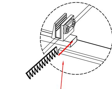
Keep the luna rail be parallel with the pivot bracket and then cut down the excess part.
