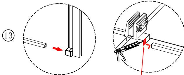
Add dab of silicone to the joint where luna rail and pivot bracket meet.
