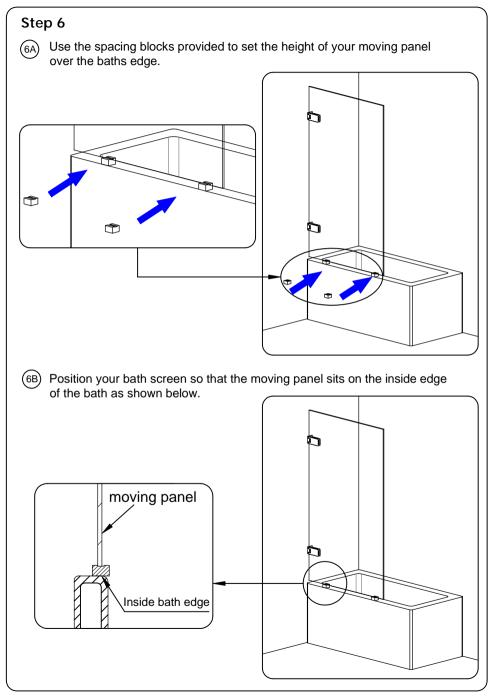
(6C) When you are happy with the position mark the fixing positions of your wall hinge making sure that your moving panel is kept plumb.
