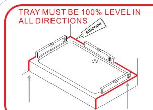
Ensure the shower tray is level in all directions and is properly sealed to the wall. The wall must be tiled down to the top edge of the tray. **Do not angle out bottom tile.**
