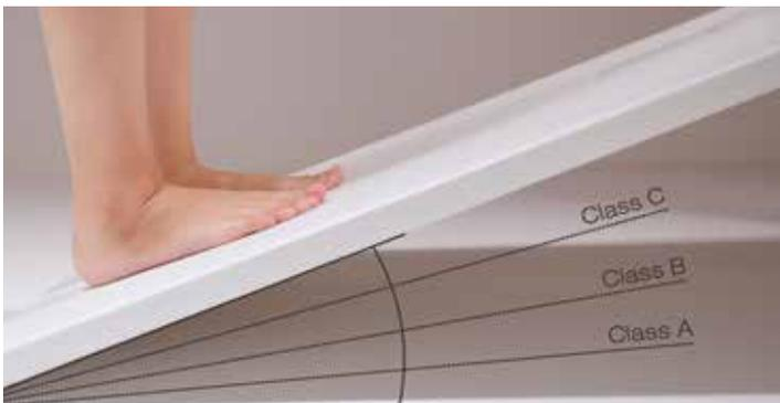
Exceeds Class C for DIN 51097 - Barefoot ramp test.
