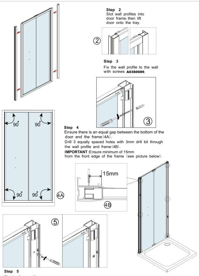
Fix the frame with screws **SPOST4**.
